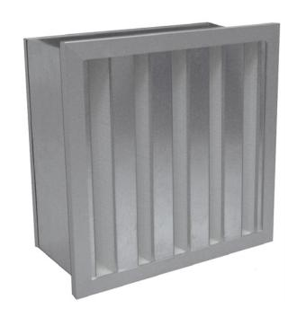
AstroCel III is a heavy duty, high efficiency particulate air filter (HEPA) designed for both Constant Air Volume (CAV) and Variable Air Volume (VAV) systems. The AstroCel III filter is made of multiple mini-pleat media packs assembled in a V-shaped configuration, into an electro-galvanized steel housing with an aluminium flange at the air entry side.
